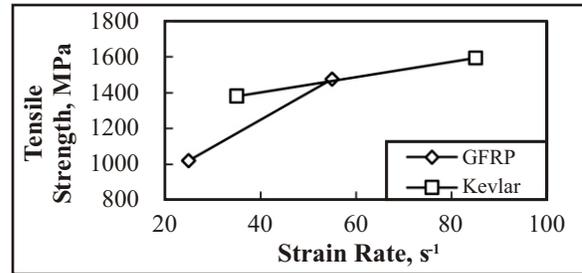
Fig. 9. Strain rate effects on Tensile Strength
