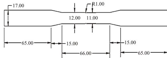
Fig. 2. Dog bone Specimen & its dimensions
