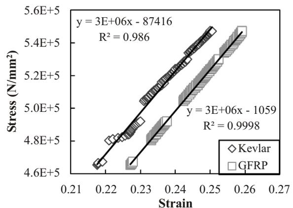
Fig. 7. Stress-Strain behavior of two polymer composites
